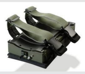
The EDM can be comfortably attached to a pilot's thigh using the straps on the back of the unit.
