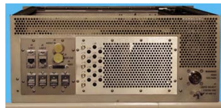
Figure 4. The rear panel includes all analog signal connections and can be customized to suit the application requirements.
