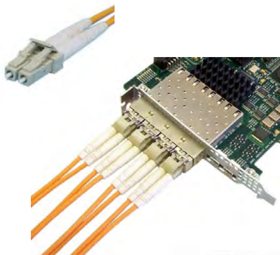
Example Optical SFP Connection to Investigator
